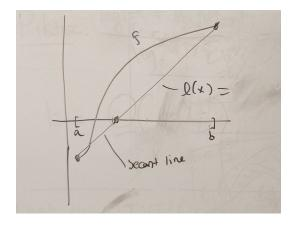
Exercise: what is l(x)?// Secant method://  $x_0 = a$   $x_1 = b$  k = 2while true:  $x_k = x_{k-1} - f_k(\frac{x_k - x_{k-1}}{f_k - f_{k-1}})$  # check if  $|x_{k+1} - x_k| < tol$ Question: time complexity?
